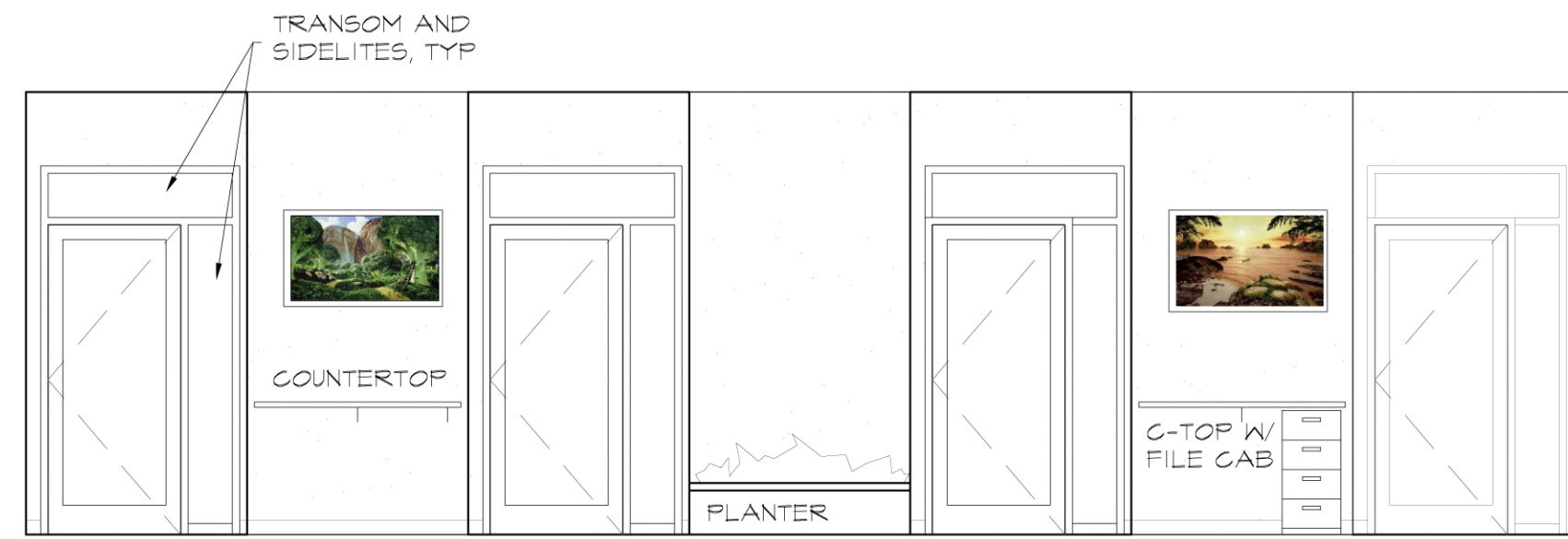
INTERIOR ELEVATION: ANGLED CORRIDOR WALL SCALE: 1/4" = 1'-0"
